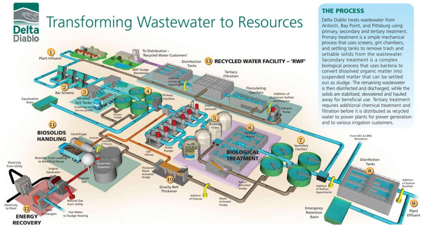
Figure 1: Delta Diablo Wastewater Treatment Plant
