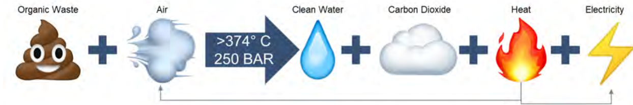
Figure 6-16 Super Critical Water Oxidation Process Concept
