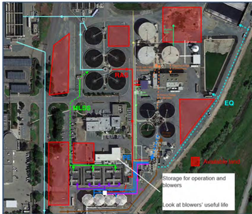
Figure 7-1: Proposed Expansion Areas at the WWTP
