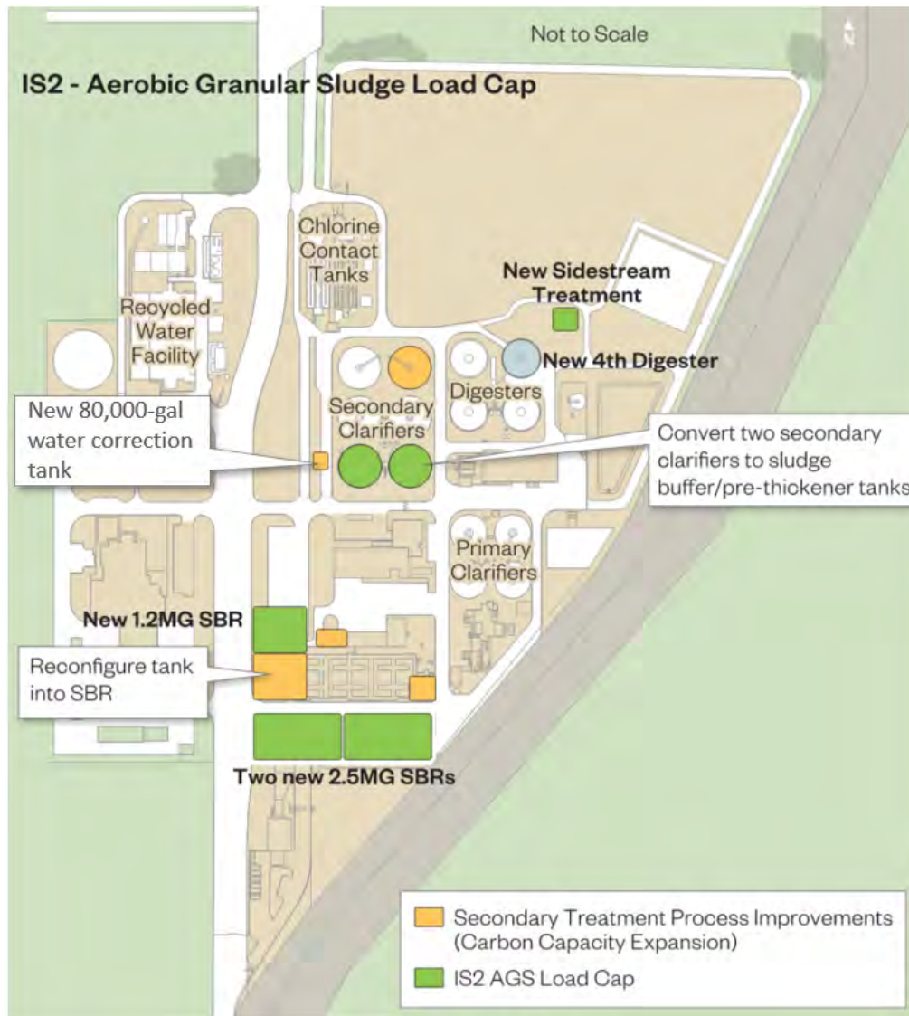
Figure 6-8 Integrated Solution 2 AGS Load Cap Required Infrastructure
