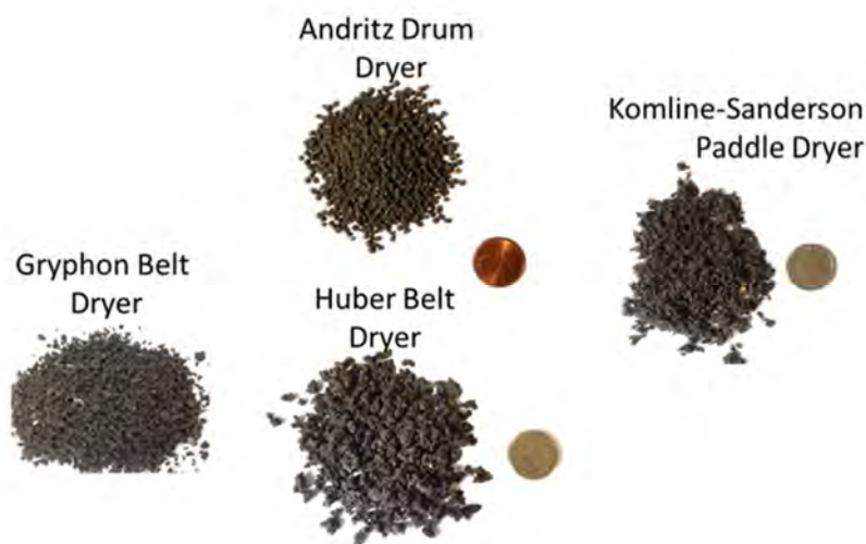
Figure 6-13 Thermal Dryer Products
